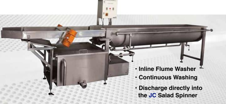
The **JC Salad Flume** Washer is for the continuous washing of salad and vegetables. With its 11 angled and 3 straight nozzles and a stainless steel vibratory deck to remove excess water
